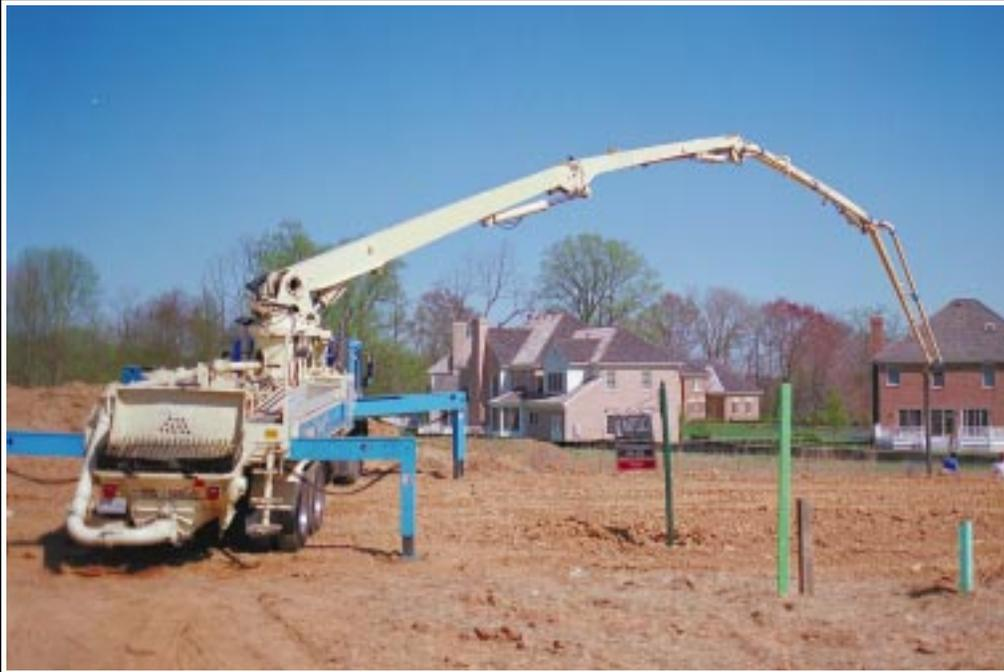
Use the proven **four section roll and fold boom** to reach in, out, down, over and under. The possibilities are endless and the results impressive when you snake this boom into buildings, under bridges, and into excavations. Low folding height of 25'-4" allows the boom to be used in enclosed settings.
