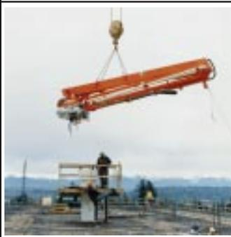
The Schwing 32-meter gains added versatility with the optional quick disconnect feature. Contractors use the truck-mounted pump with placing boom in its conventional mode for part of a day on slab pours or other ground level placements and quickly remove the boom (with the aid of a tower crane) for remote placements later in the day.
